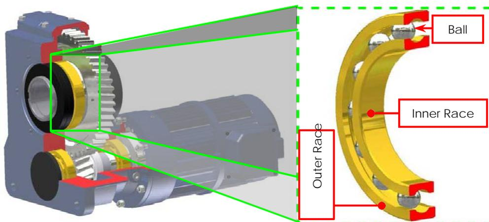
As noted, a bearing is a *low-friction* device, it is not friction-free. As one race rotates about the other race, the balls (or rollers) likewise rotate/slide within the race. The rotating/sliding action of the balls (or rollers) creates friction between these bearing components thereby creating an additional avenue for energy loss.
