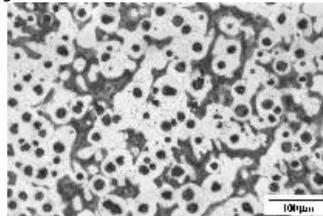
Figure 4. Grey Cast Iron Grain Structure
